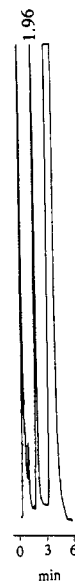
Figure 1. GC-ECD chromatogram for profenofos residues in a fresh washed tomato sample 1 week after pesticide application. The retention time for profenofos is 1.96 min.
